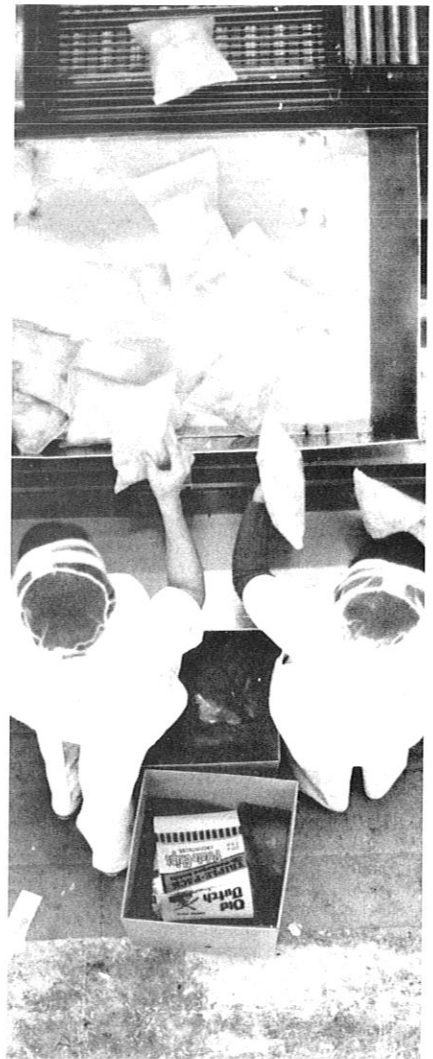
Above, the chips are separated by a chip sizer before entering this conveyor above the packaging lines. Note how the chips are channeled through a seasoning drum which applies the seasoning powder to the chips (see arrow).
