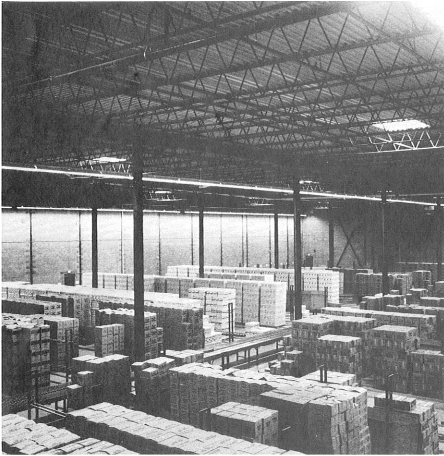
Above, the shipping area features a conveying system to bring product from the adjacent warehouse to load the route trucks from individual docks.
